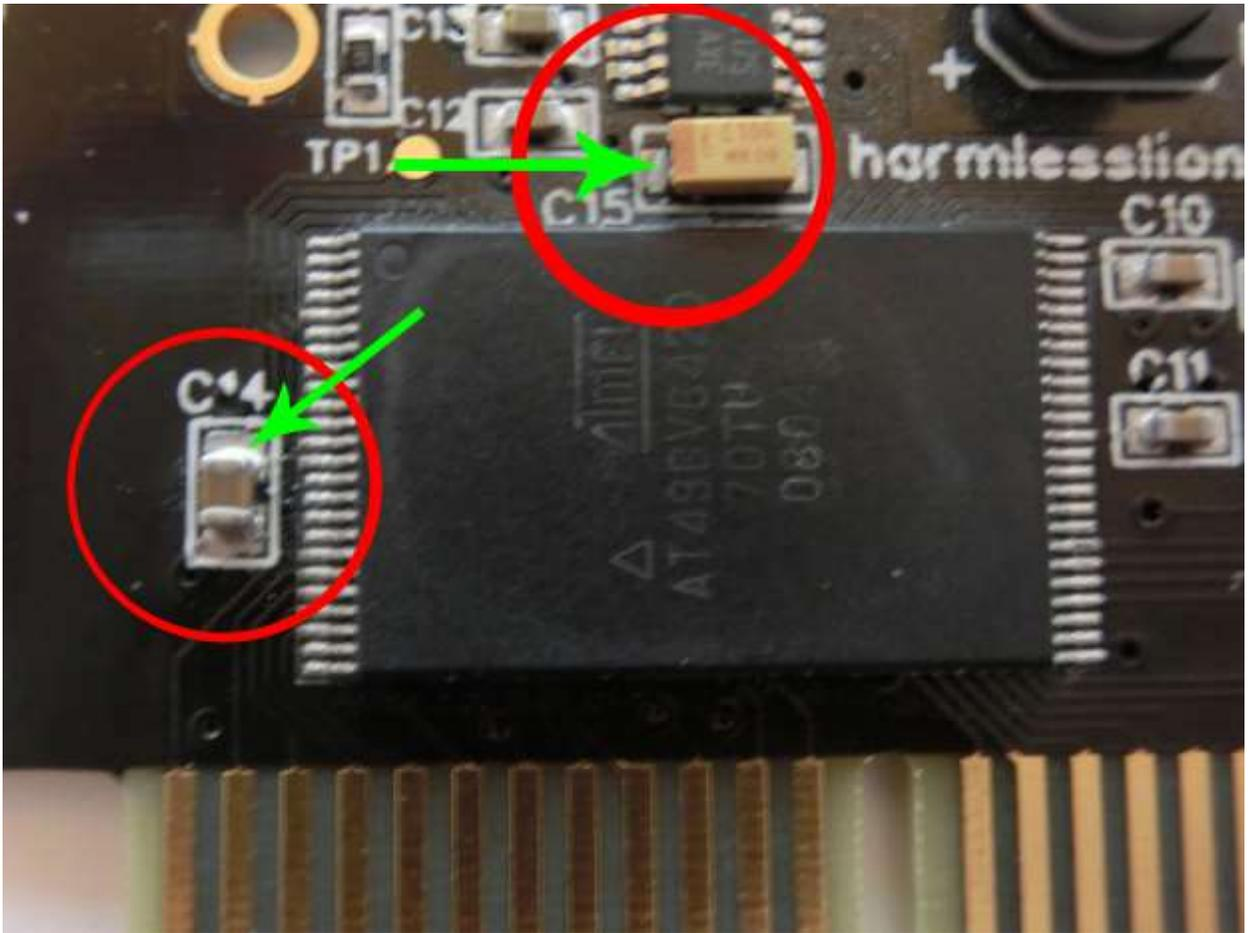
8. Attach a jumper wire connecting the two capacitors as shown below. Feel free to do a better job than I did. ;) Note that attaching to the correct side of each capacitor is very important. Be careful not to spill solder onto neighboring parts.
