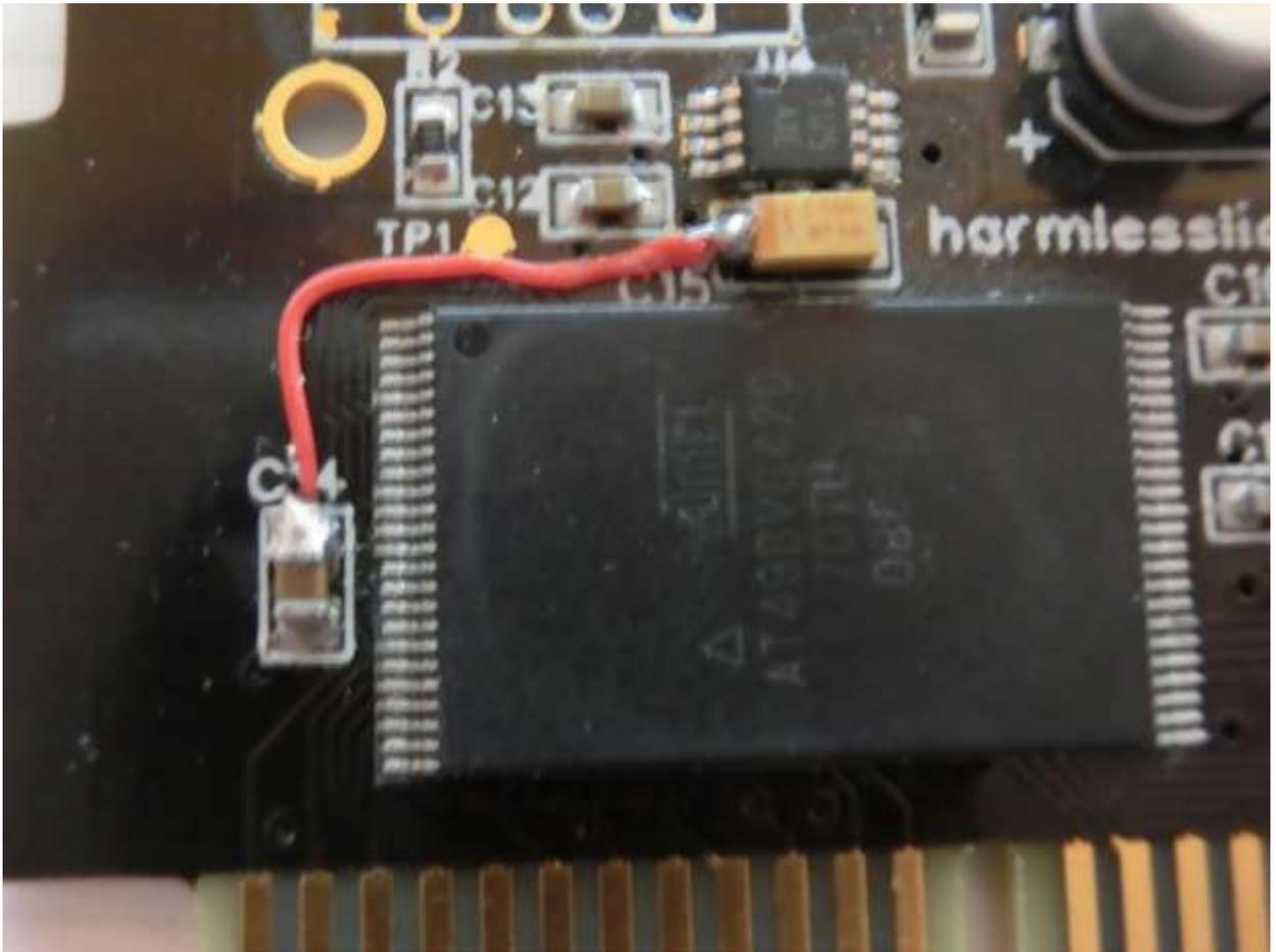
9. Use an ohmmeter to verify connectivity. This connects the regulated 5v to the programming pin.
