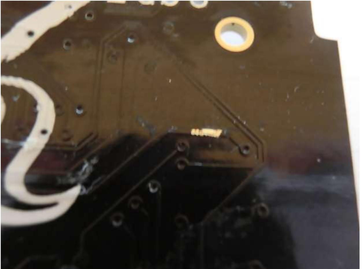
4. Remove a portion of the copper trace to break conductivity. The easiest way is to make two cuts across the copper and remove the copper between the cuts. Again, be careful not to nick other traces, do not cut deeply into the PCB itself, and do not cut yourself.
