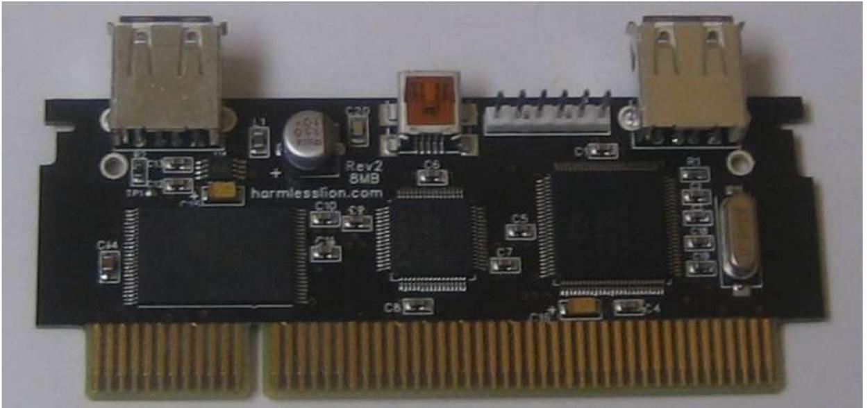
7. Identify C14 and C15 as in the following picture. The arrows show the sides you must attach to.
