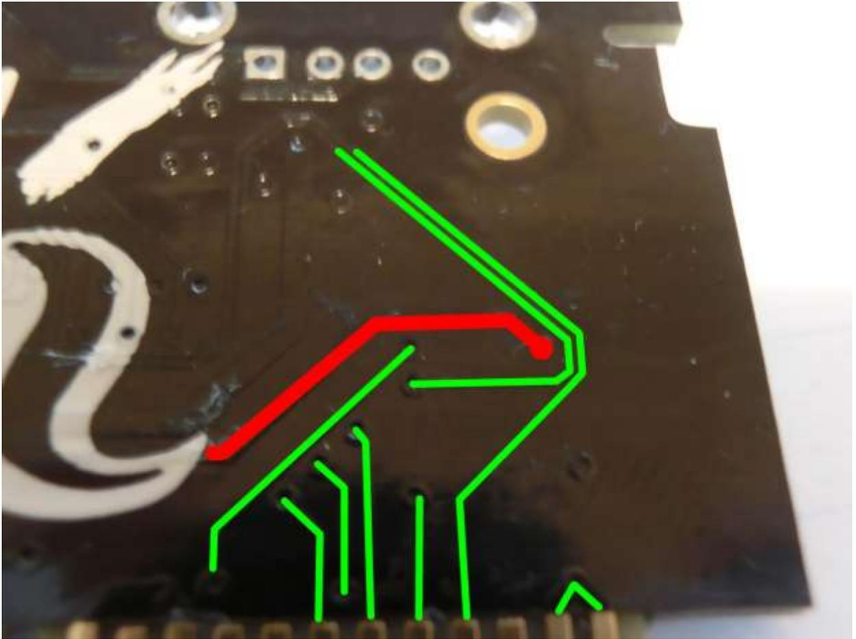
3. Using a sharp knife, carefully scrape off some of the solder mask to expose the copper beneath. Be careful not to nick other traces and do not cut yourself.
