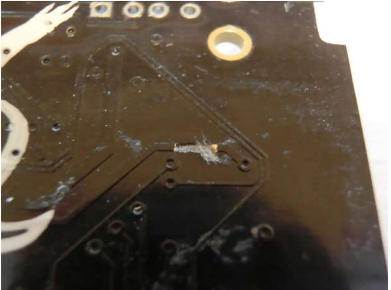
5. Use an ohm-meter to verify no conductivity across the cut trace. This disables the 9v feed to the flash chip.
